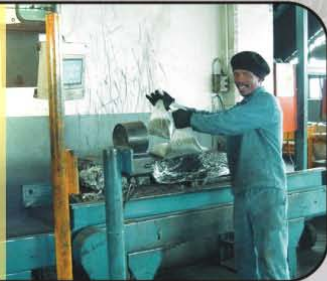
Preparing a batch of raw rubber for mixing
