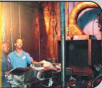
At the end of the conveyor, the raw rubber is fed into the mixer
